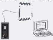
Connection of ConfigMate 4590 to a PR 4000/9000 device:
