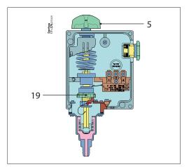
The range is set by using setting knob (5). Tools must be used to set switches fitted with seal cap. To read the range scale front cover must be removed. On the units with adjustable differential, differential disc (19) must be set after removing front cover. For proper adjustment differential roller must be used. Detailed information can be found in RT data sheets, non-explosive version.
