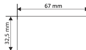
Panel cut-out dimensions
