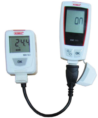
Female USB / male micro-USB adapter (reference: KNT-A)
