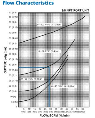
Example: The 0-60 psig range unit set at 30 psig will flow 28 SCFM with an 8 psig rise in pressure above the set point. all values assume relief flow is to atmosphere.
