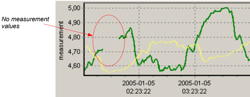
Fig. 3.10. Interruption in the graph (e.g. sensor fault)
